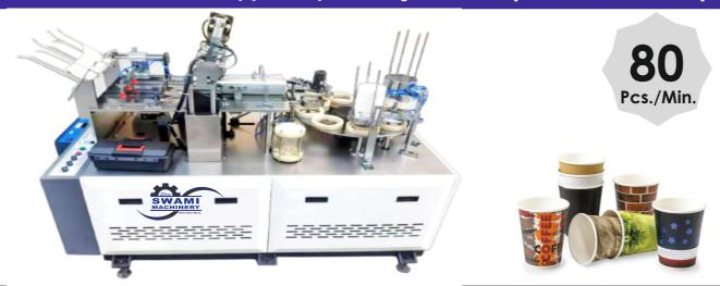
Cup Size2-12 OZBowl Size35 OZ (Mould Exchangeable)Paper Material180-450g/m Single/Double PE
